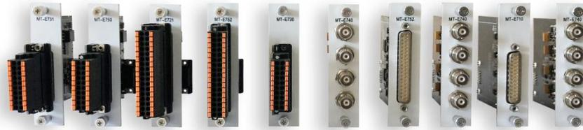
MT provides more than 20 E Series modules for measurement, control, and communication applications. E Series modules can connect to any sensor or bus and allow for high-accuracy measurements that meet the demands of advanced data acquisition and control applications.
