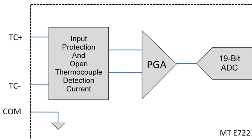
Each channel passes through a differential filter and then is multiplexed and sampled by a 19-bit ADC. The channels share a common ground, COM, that is isolated from other modules in the system.
