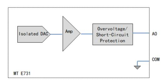
Each channel has a digital-to-analog converter (DAC) that produces a voltage signal. Each channel also has overvoltage and short-circuit protection.
