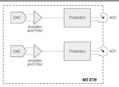
The Delta-Sigma DAC has a resolution of 24 bits and can update at a maximum rate of 192kS/s.The output stage of the MT E735 with BNC is single-ended, the AO- is terminated to GND.The outputs of the DAC are buffered, conditioned, and filtered before reaching the module conncetors.
