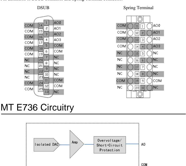
Each channel has a digital-to-analog converter (DAC) that produces a voltage signal. Each channel also has overvoltage and short-circuit protection.
