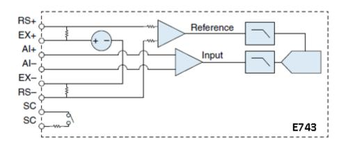
Each channel on the MT E743 has an independent 24-bit ADC and an input amplifier that enable you to sample signals from all four channels simultaneously
